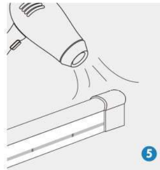
Dry the plug with heat gun until the silicone is firm
