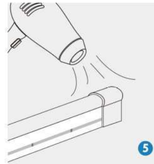
5 Dry the plug with heat gun until the silicone is firm
